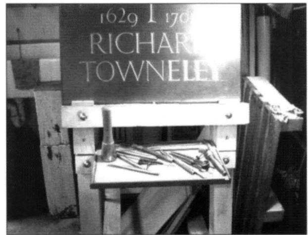
Fig.4. Work in progress with tool tray mounted on the easel.
