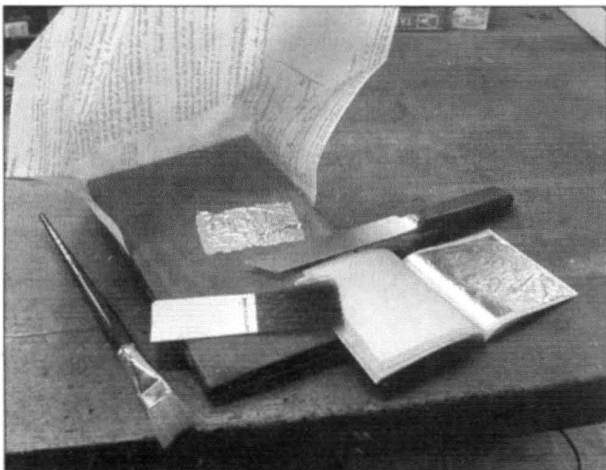
Fig.10. Gilder's tools; the draught-screened cushion with a portion of gold leaf on it ready for cutting, cutting knife, gilder's tip, book of gold leaf and soft brush.
